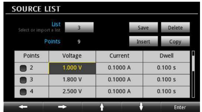
Figure 7A. Create an output sequence using the List setup screen.
