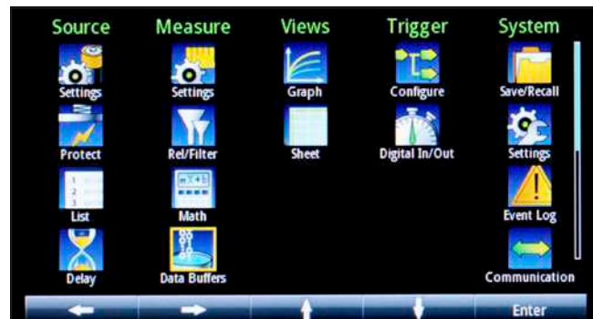
Figure 4. Access the full functionality of the Series 2280S supplies from the main menu.
